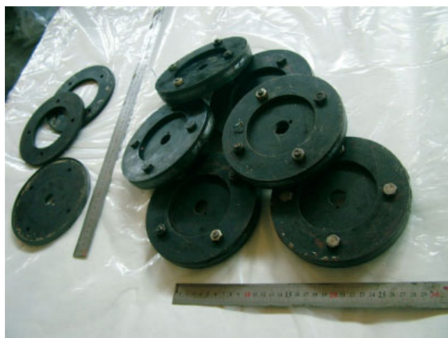
Figure 4 The NOL hoop specimen for tests. [Color figure can be viewed in the online issue, which is available at www.interscience.wiley.com .]
